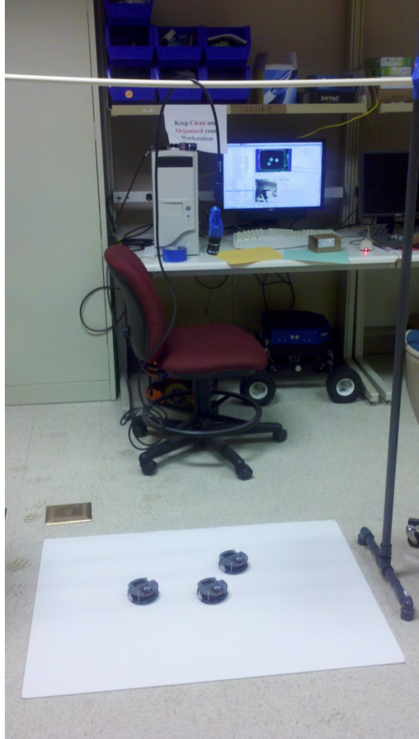
Figure 7 The Global Vision System Consisting of Camera and a Linux Computer running the SSL-Vision Software
