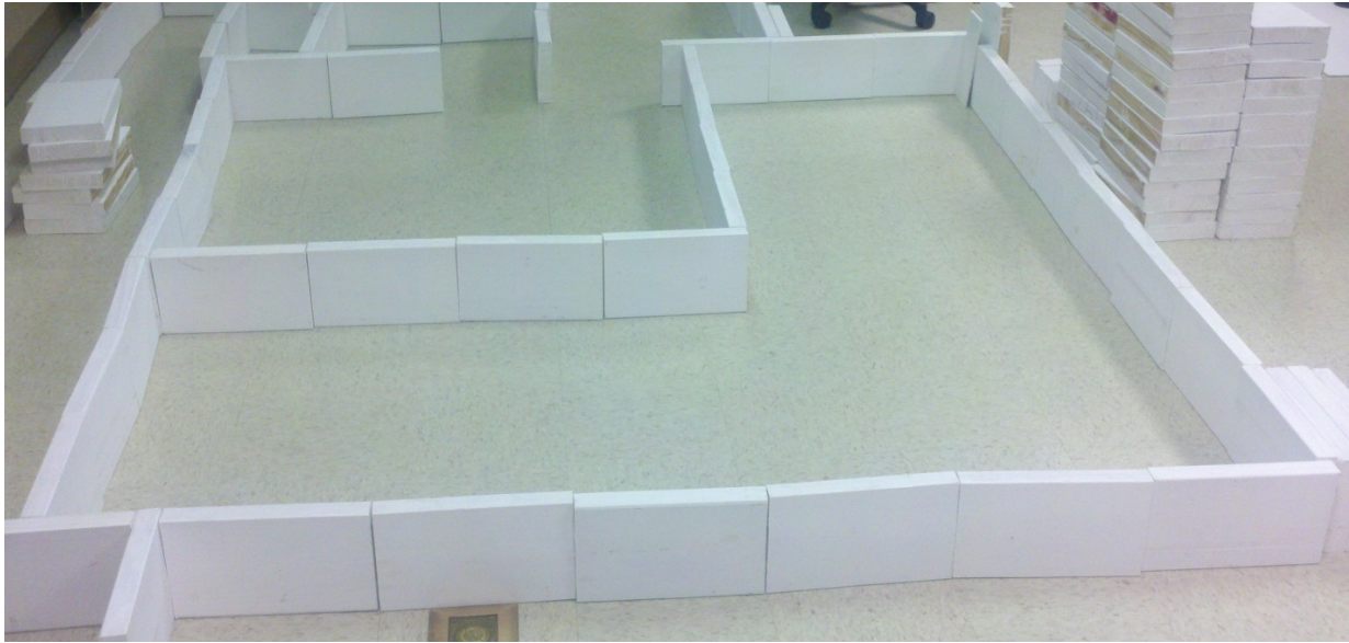
Figure 2 An L corridor used to test the SLAM algorithm
