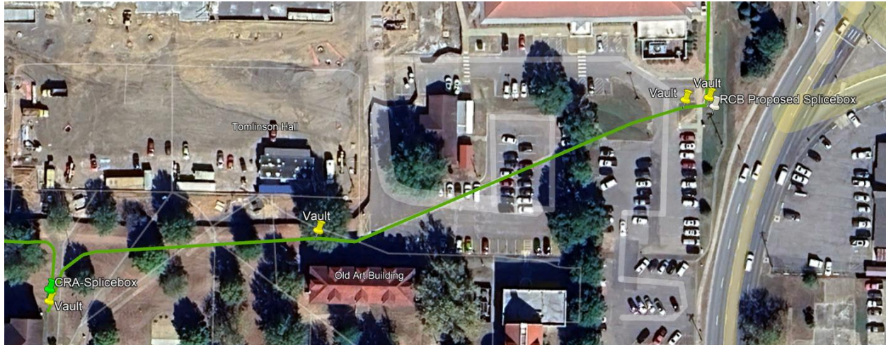
Figure 4: The rough path for the first required fiber run between the Crabaugh splice box (labeled as “CRA Splicebox” with a green pin) and the new Brown Hall splice box (labeled as “RCB Proposed Splicebox with a white pin).
