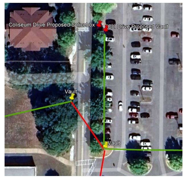
This is an acceptable alternative assuming there is a cost savings (bearing in mind if Option B is chosen, fiber would then be run in this new path and would require an extra few hundred feet of length to go South first before crossing the road) or improves the ease of the bore in some way.
